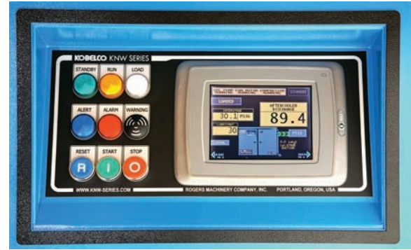
Figure 1-26 PLC operator interface and monitor. Source: Courtesy Rogers Machinery Company, Inc.
