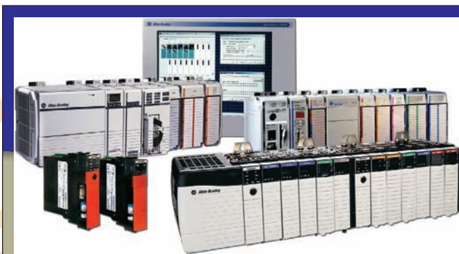
Figure 15-1 Programmable automation controllers (PACs). Source: Image Used with Permission of Rockwell Automation, Inc.
